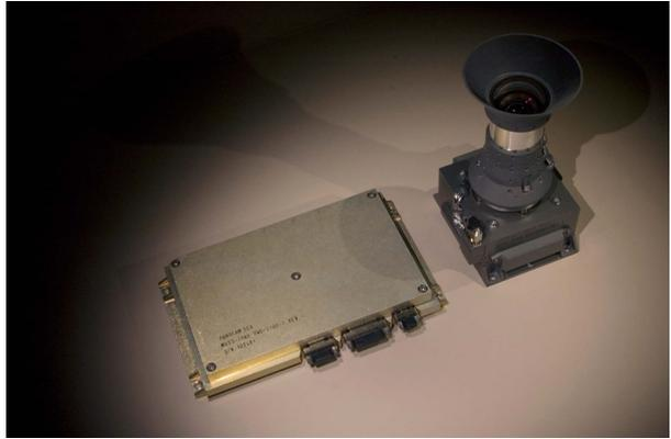
**Fig. 2** The Junocam camera head is mounted to the side of the spacecraft, with its boresight perpendicular to the spacecraft rotation axis
